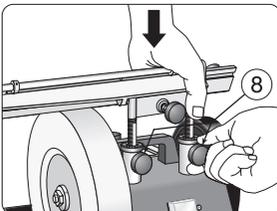
Lock the support plate – while it is pressed down – with the two locking screws (8).
