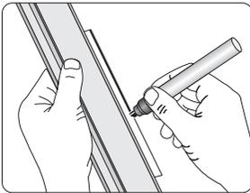
Colour the grinding bevel with a marker pen so that you can see where the grinding occurs when setting the edge angle.
