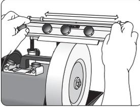
Grind by moving the holder with even pressure from side to side between the side stops.
