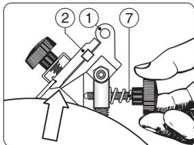
\* You can sharpen blades up to 310 mm in one step, but make sure to use the Stone Grader SP-650 during sharpening so that the stone maintains a flat surface. (The small uneven wear that occurs during sharpening will otherwise make it difficult to sharpen the blade at the edges.)
