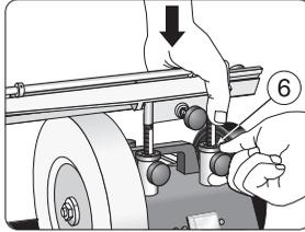
Press down the grinding jig while locking with the locking screws so that the two wheels (6) rest on the base without any gap.
