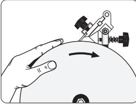
Check the angle setting by turning the wheel by hand. The wheel should make marks on the whole bevel, from the tip to the heel.
