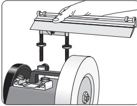
Remove the Universal Support and place the support in the sleeves of the machine. If required, remove the honing grinding wheel.
