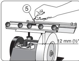
Place the blade holder on the support. Set the grinding length to the length of the blade to ensure that the blade does not run off the edge of the stone during grinding. This is done by adjusting and locking both stops (5). Blades longer than approx 270 mm (10 1/2"), you move in the holder and grind in two steps.\*
