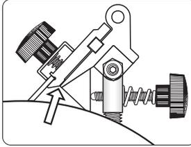
You must grind until the blade holder rests against the support along the whole length. Grind the other blade with the same setting.
