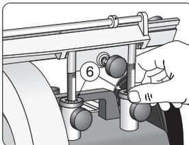
Make an initial height setting with the wheels (6). Set the edge angle with the adjusting screw (7). Make fine adjustments to the height with the wheels (6). The bevel should now lie flat on the stone and the holder (2) should touch the support (1).
