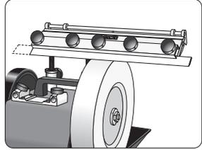
For longer blades more than 270 mm (10½"): Move the blade in the holder and grind in two steps. Make sure that the back of the blade rests on the stop.
