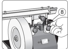
Set the grinding depth by raising the wheels (6). Turn the wheels equally in order to retain the parallel setting. The grinding depth is shown on the two wheels (6) which are graduated for each 0.1 mm (0.004"). The numbers on the wheels (6) do not need to be synchronised.
