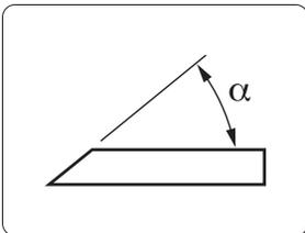
Grind the blade at exactly the original edge angle ( $\alpha$ ).
